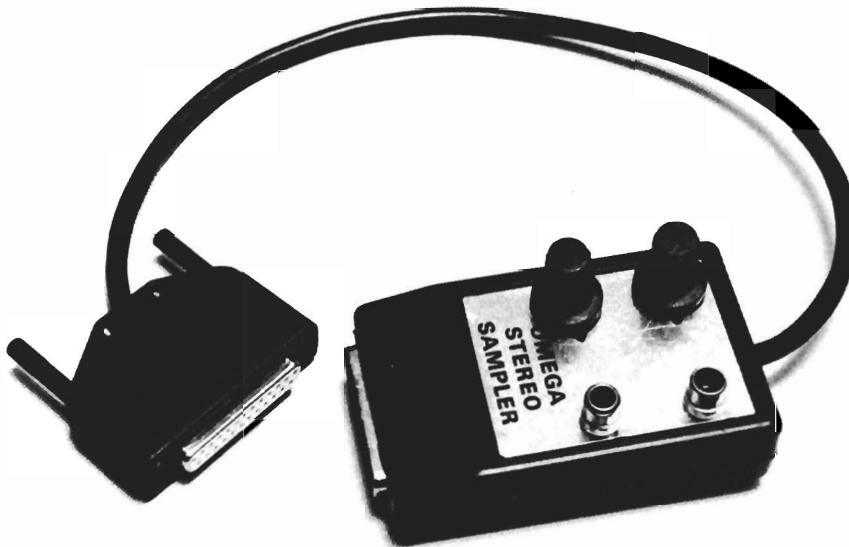
The Omega Stereo Sampler plugs simultaneously into the parallel and serial ports
